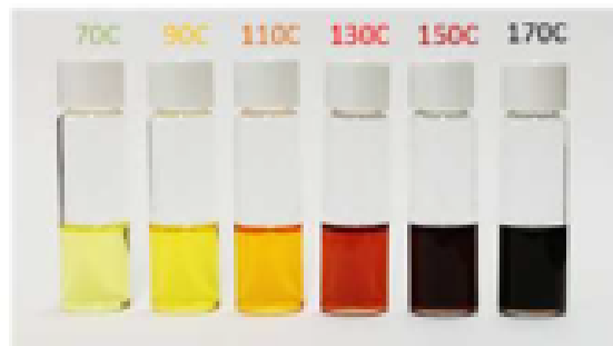
Figure 3.6 Toluene solutions of Zn-CIS NCs synthesized at different growth temperatures [33]
