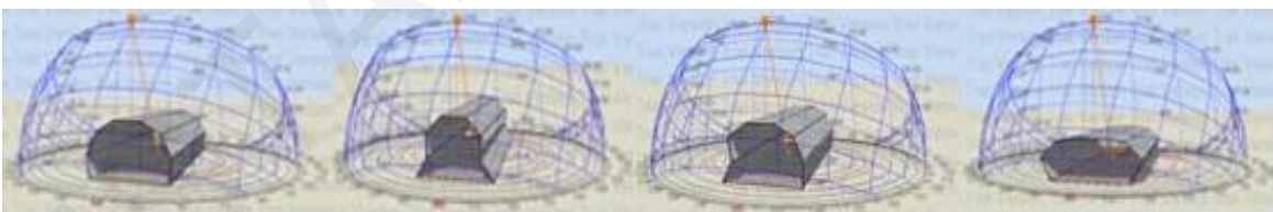
Figure 5.11 Sweden's sun path diagrams on 21st of June at 12:00 am (site orientation: 0°)
