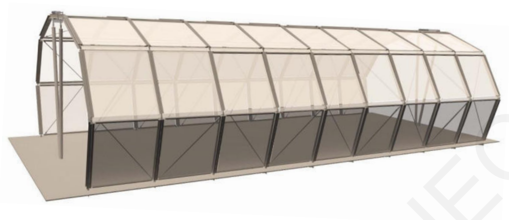
Figure 3.14 Spatial structure with vertical reconfigurability and ETFE membrane
