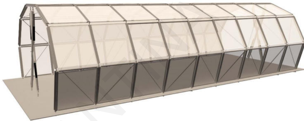
Figure 3.15 Spatial structure with horizontal reconfigurability and ETFE membrane
