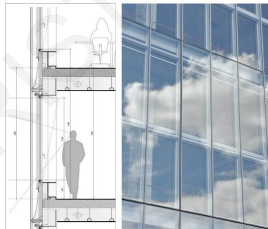
Figure 5. New Courthouse in Paris by Renzo Piano Building Workshop Façade Cross Section (left) [4] and Façade External View (right) [5].
