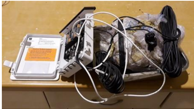
Figure 50. Block samples with inserted monitoring sensors of matric suction (TEROS 21) and volumetric water content (TEROS 12) and data recording through ZL6 datalogger.
