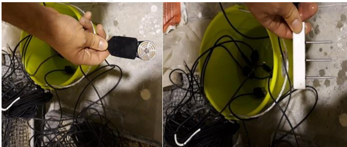
Figure 49. Preparation of TEROS 21 matric suction sensors (placed in water for 24 hours) and TEROS 12 volumetric water content sensors prior to installation.
