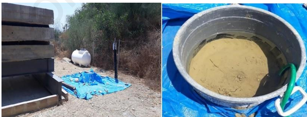
Figure 20. Wetting area protection with plastic sheets to prevent atmospheric evaporation (left) and initialization of the field wetting experiment (right).
