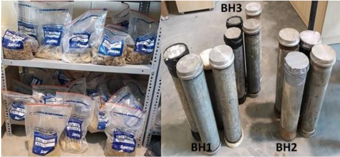
Figure 13. Bulk and undisturbed U100 samples from the boreholes.
