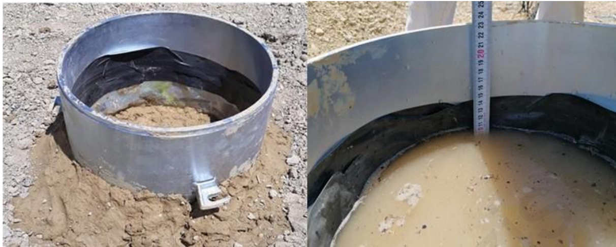
Figure 35. Wetting experiment configuration at Site 3
