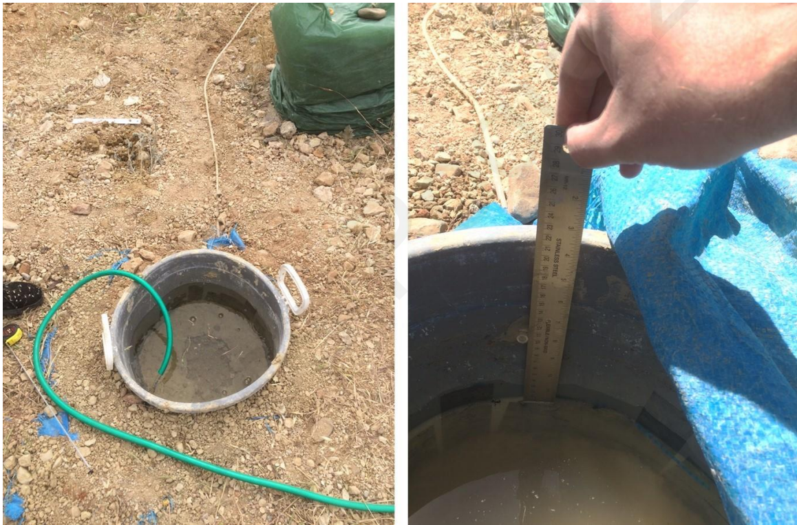
Figure 28. Initiation of field wetting experiment (left) and plastic drum with overflow (right).
