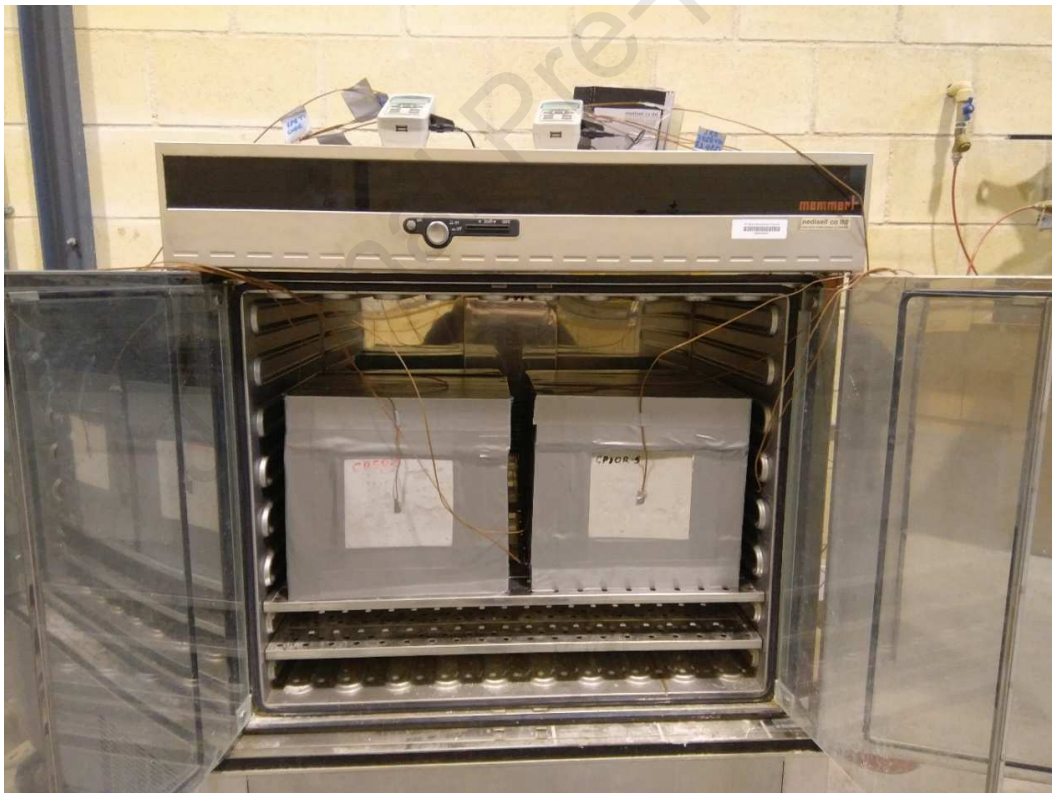
Figure 4. Schematic representation (a) and photograph (b) of the test set-up implemented to investigate the response of mortar plate samples to temperature variations in laboratory-controlled environment.
