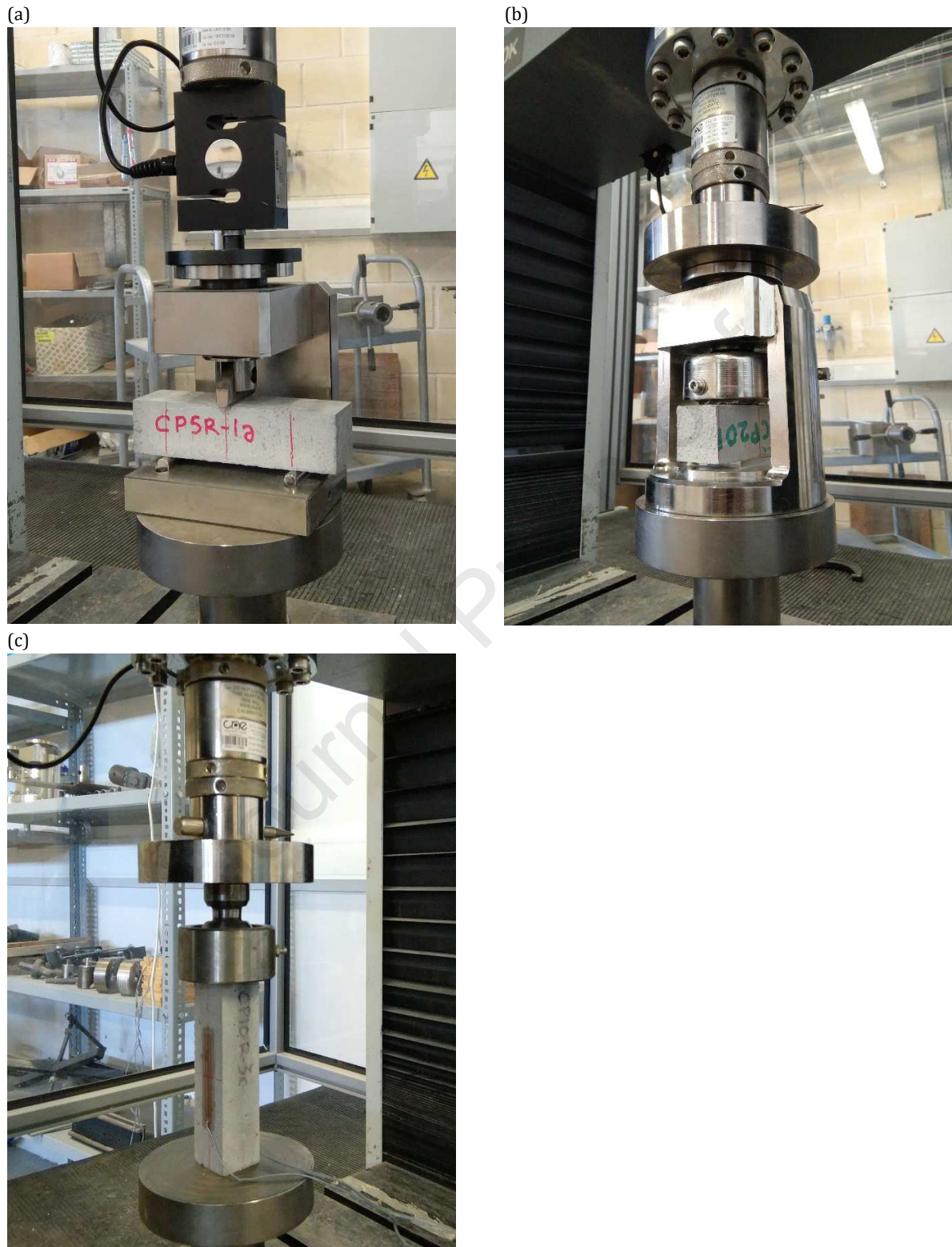
Figure 3. Test set-ups used for the implementation of loading tests: (a) Three-point bending of mortar prims and (b) compression testing of half-prim as per EN 1015-11 [33]; (c) Uniaxial compressive loading tests with deformation monitoring on mortar prims fitted with strain gauges as per EN 13412 [34].
