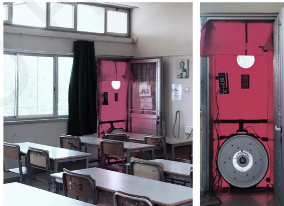
Figure 10.16. Blower door test for the determination of airtightness of the building.
