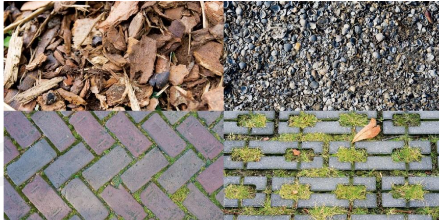
Figure 7.5. Indicative photos of water-permeable materials and surfaces [387].
