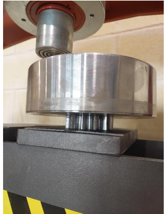
Figure 37: Positioning of joined parts in the manual press
