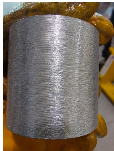
Figure 63: Surface of sanded aluminium
