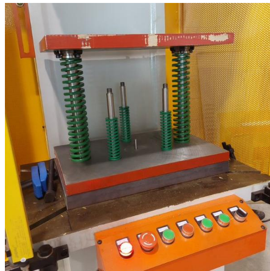
Figure 35: The top plate is secured on the guide pillars with two guide bushes
