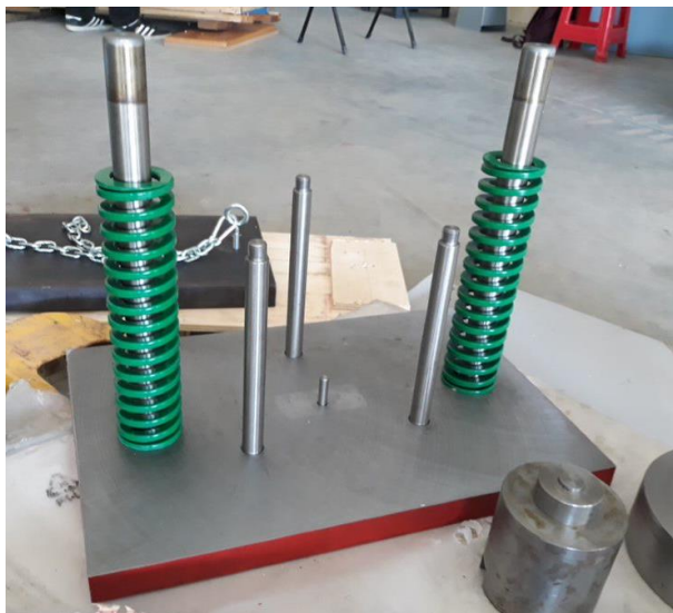
Figure 35: Base plate with two basic toolset guide pillars with springs, three forging toolset guide pillars and pin in the centre for alignment
