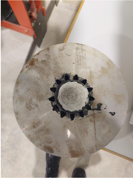
Figure 36: Removal of joined part, die and counterpunch
