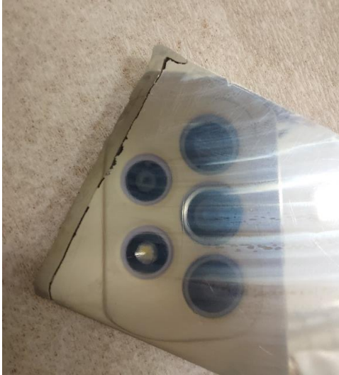
Figure 61: The polished section of gear 2
