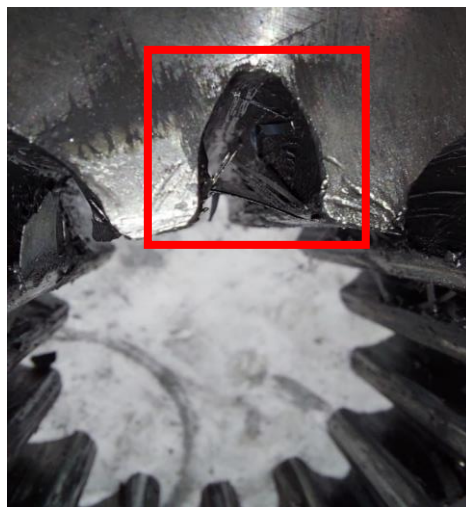
Figure 38: Oxide residues on the die
