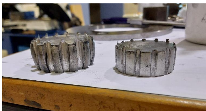
Figure 29: Side view of forged annealed (left) and non-annealed (right) aluminium parts
