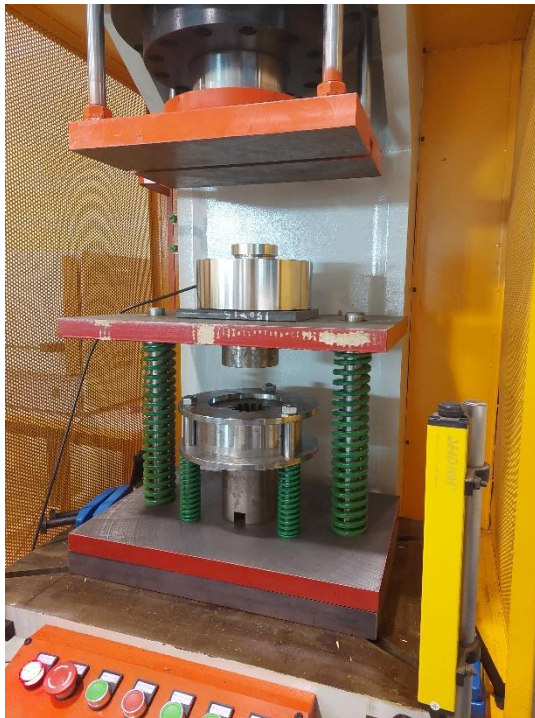
Figure 55: The Load Cell is placed on the top plate
