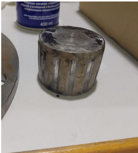
Figure 74: Gear teeth could not be formed due to material flowing over the die
