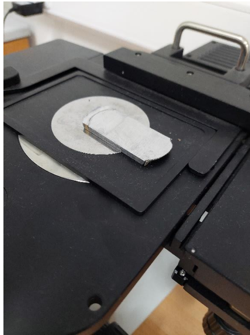
Figure 65: Sample placed on the microscope with the polished side facing down
