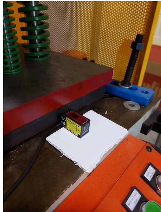
Figure 55: The Laser Distance Sensor is placed on the bolster
