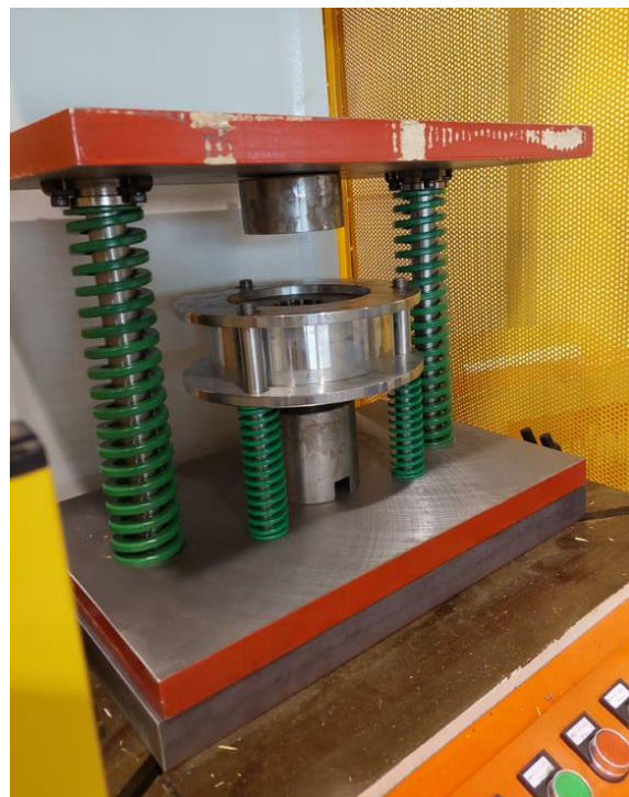
Figure 53: The punch is fastened at the downside of the top plate
