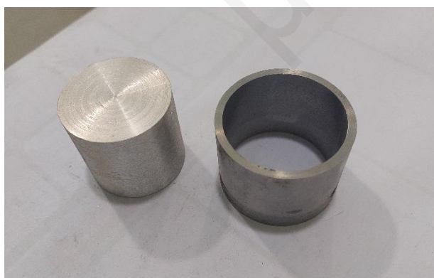
Figure 59: Un-bonded steel outer ring and aluminium inner cylinder
