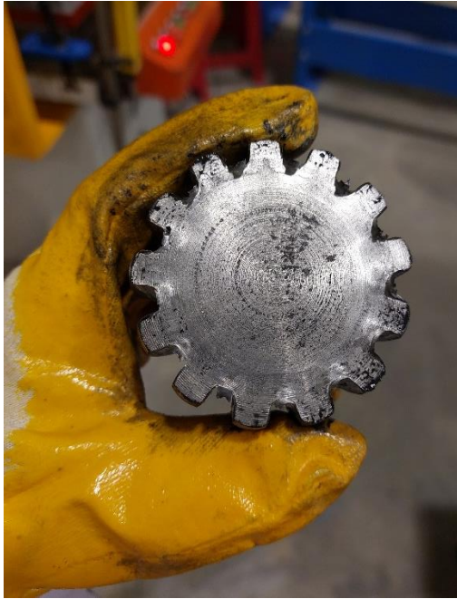
Figure 30: Forged annealed aluminium part
