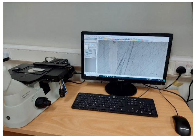
Figure 64: High resolution images of the interfaces could be obtained from the computer connected to the microscope
