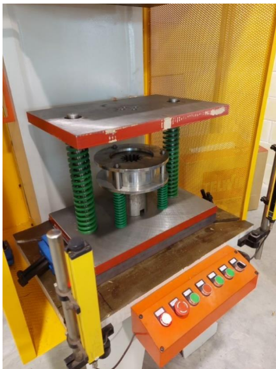
Figure 53: The second ring is placed on top of the die
