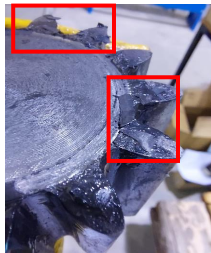
Figure 39: Oxide flakes on the counterpunch
