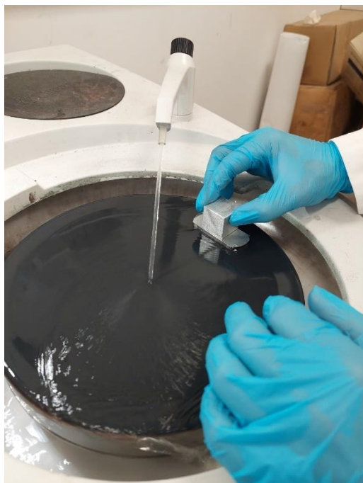
Figure 59: Polishing of the sample
