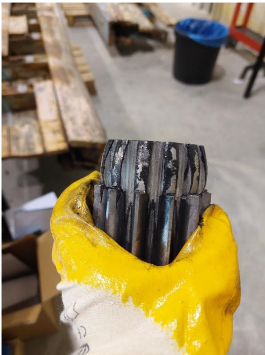
Figure 34: The forged part and counterpunch are joined due to flash
