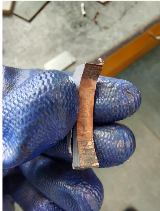
Figure 54: Detached outer layer of gear 4 with copper film
