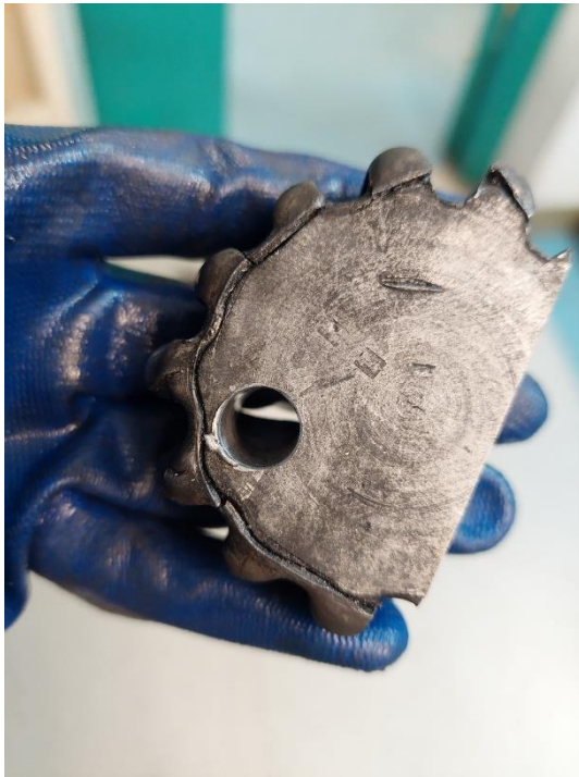
Figure 51: Off-centred hole drilled on gear 2
