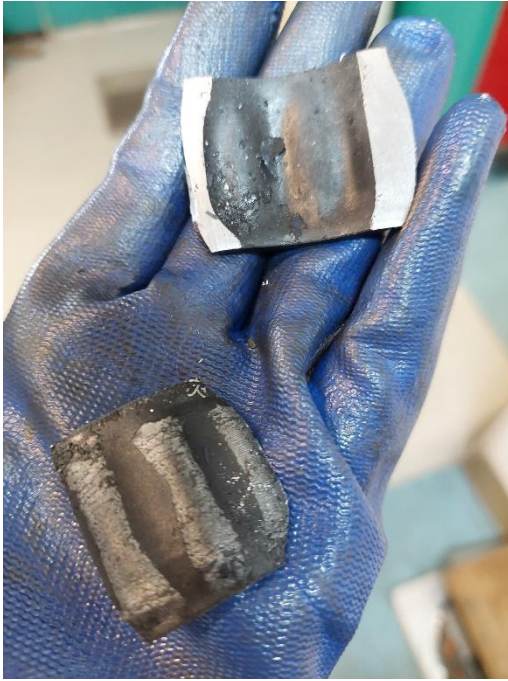
Figure 53: Detached pieces of gear 1, with oxide flakes observed on the outer layer
