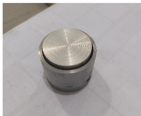
Figure 59: Assembled steel ring and aluminium cylinder
