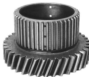
Figure 1: Welding of spur and helical gear [8]
