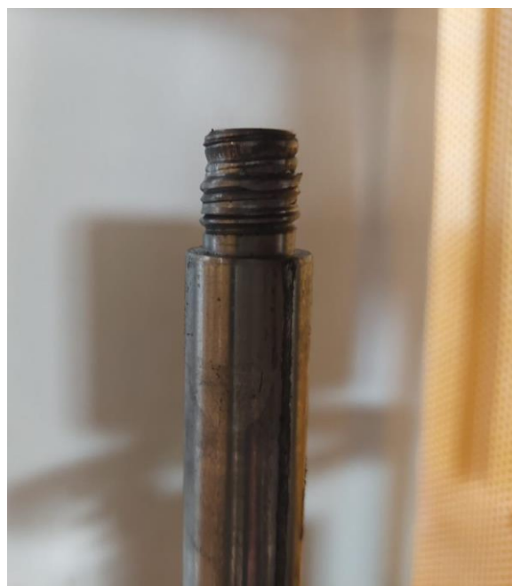
Figure 76: Deformation of pillar
