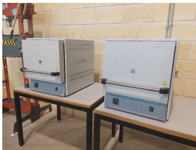
Figure 57: The two SNOL Muffle Furnaces
