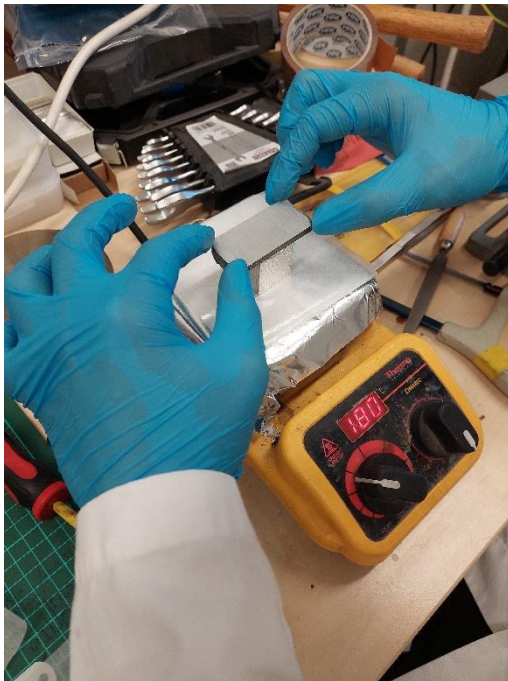
Figure 57: Heating of the metallic cube and securing the sample with wax
