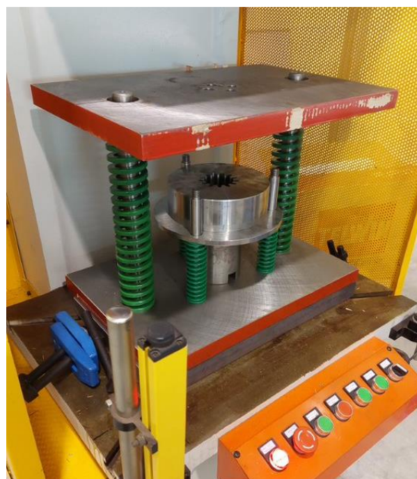
Figure 45: Placement of die on top of the ring
