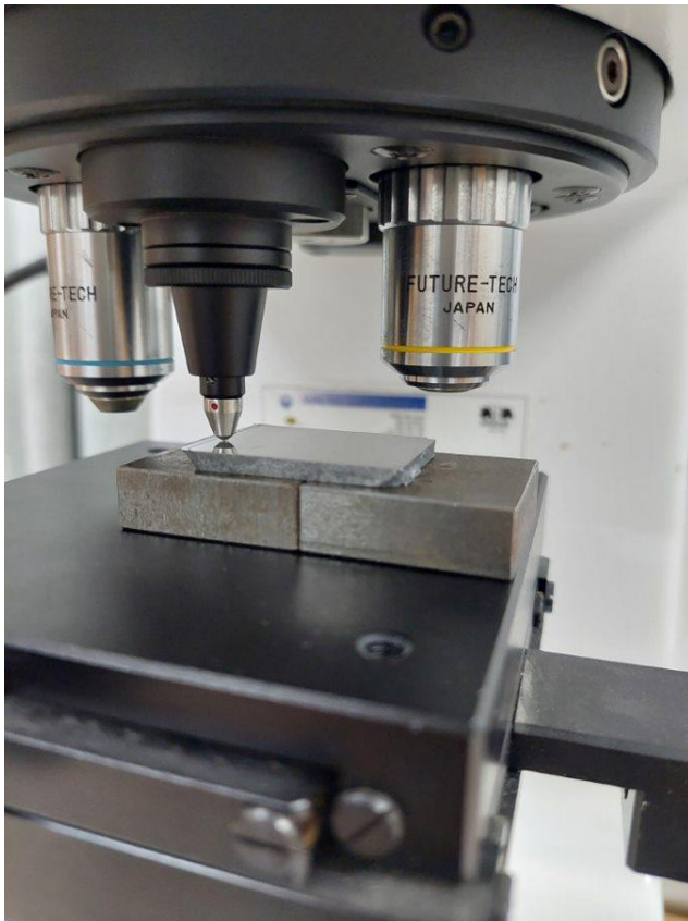
Figure 72: Vickers indenter on the section of gear 2
