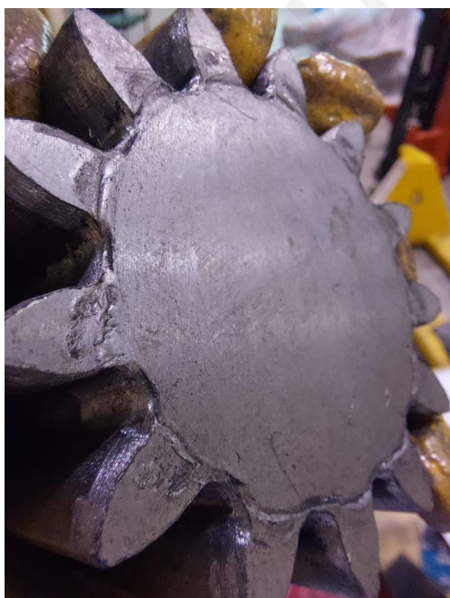
Figure 75: Damage on counterpunch
