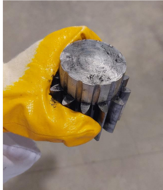
Figure 31: Forged non-annealed aluminium part
