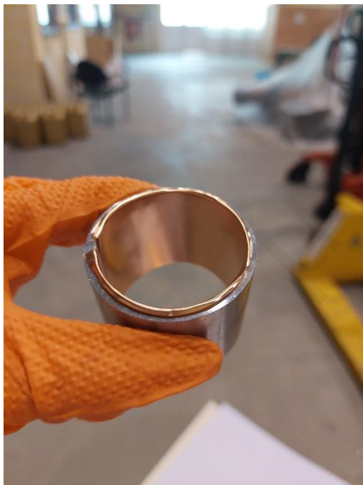
Figure 32: Copper film wrapped on the inside surface of the AA6062 ring
