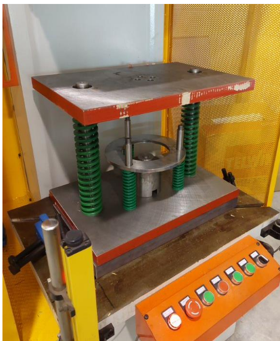
Figure 43: Placement of alignment tool and first ring through the smaller pillars
