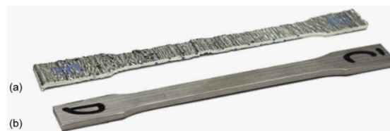
Figure 3 (a) Extracted as-built and (b) machined coupons [20].
