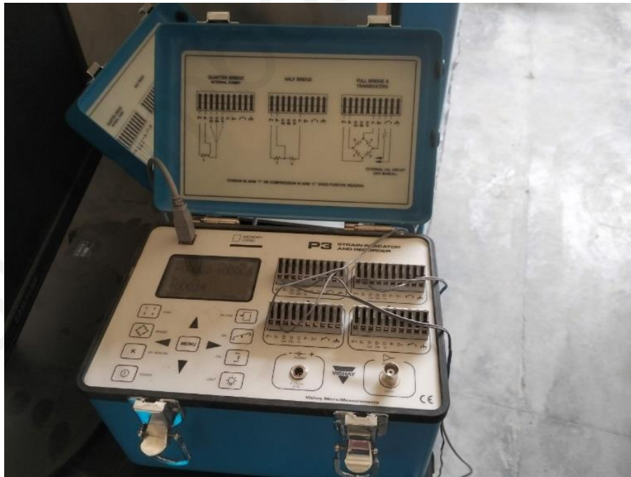
Figure 15: VISHAY 3P indicator and recorder. 4 strain gauges can be connected to measure the shrinkage in \mu\epsilon .
