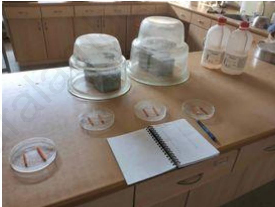
Figure 8: Setup for the sorptivity determination. The specimens were left into matrices until their temperature was stabilized.
