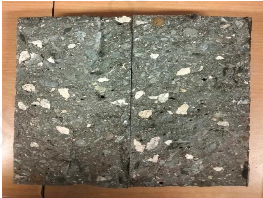
Figure 19: A specimen after the tensile failure. Some small opes can be identified inside the specimen which resulted into lower tensile strength than anticipated.
