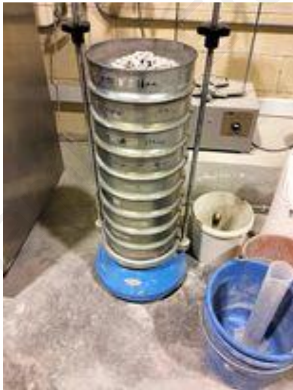
Figure 3: Sieve machine used for the determination of the size distribution of aggregates.
