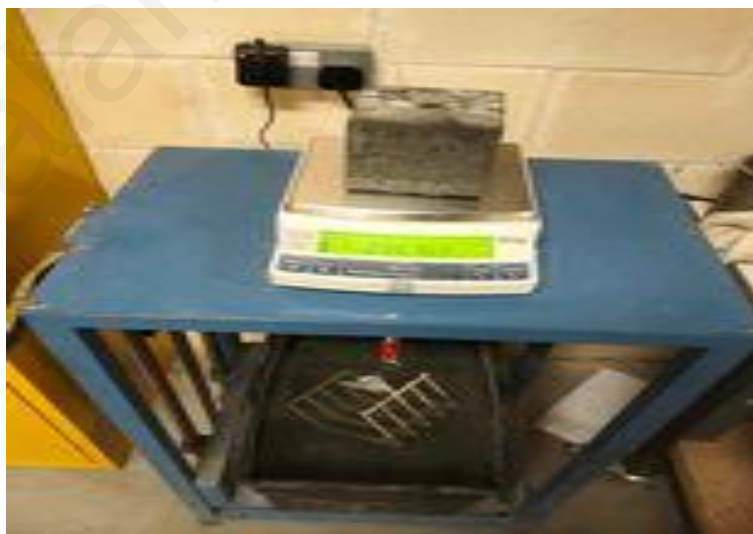
Figure 7: Setup for the determination of porosity of concrete.
