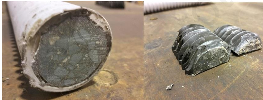
Figure 13: A section of the auto shrink specimen. The exposed concrete was covered with a water insulations substance that is used for roofs (left). The specimen from Figure 8. The specimen was cut in half to identify if the corrugations were successfully filled. The figure shows that more vibrations are needed to fully fill the corrugations (right).
