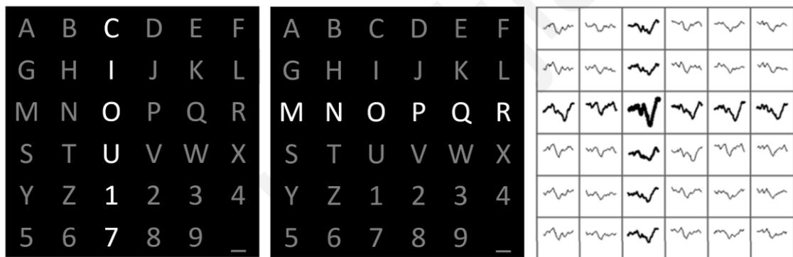
Fig. 7. An example of a 6x6 symbol P300 matrix based BCI system. The user wants to write the letter "O" by focusing on the letter. The system recognizes the correct letter because of the positive peak generated in the EEG signal 300ms after the flash [55].
