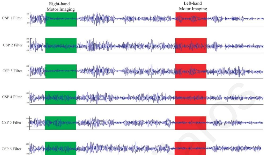
Fig. 16. EEG signals spatially filtered with the common spatial patterns (CSPs) algorithm. CSP1, CSP2, and CSP3 maximize the variance of the signals in the “imagined movement of the left hand” class (in red) while minimizing those of the “imagined movement of the right hand” class (in green). CSP4, CSP5, and CSP6 do the opposite, they maximize the variance of the “imagined movement of the right hand” class, while minimizing the variance of the “imagined movement of the left hand” class.
