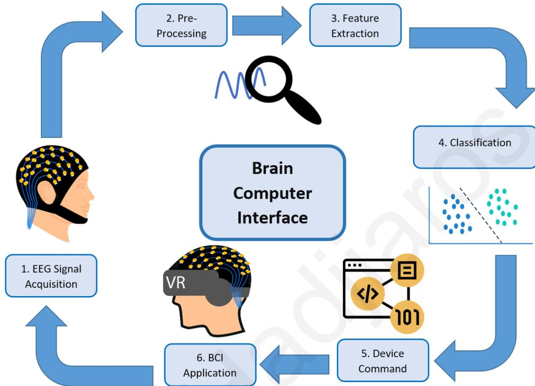
Fig. 1. Main components of a BCI-VR Gaming system. (1) raw EEG signal acquisition, (2) pre-processing of EEG signal for background noise cleaning, (3) extraction of specific application features from the clean data and selection of more discriminative features, (4) classification of the selected features, (5) decision making linked with device and command, and (6) application execution and feedback to the user.
