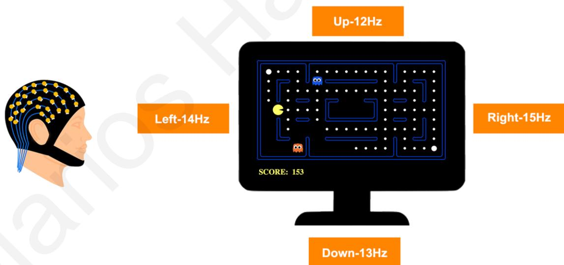
Fig. 8. SSVEP paradigm: The user moves the game character by focusing on the corresponding flickering lights. By focusing on the left flickering light, the EEG signal reflects the 14Hz stimuli and the system triggering a movement to the left [58].
