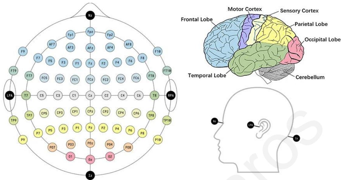
Fig. 4. The international 10-20 system labels the electrodes based on positions over the frontal, parietal, temporal, and occipital lobes, indicated by the letters F, P, T, and O respectively.
