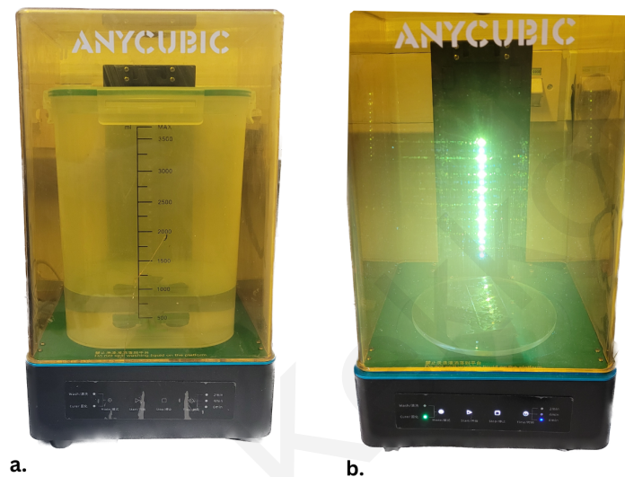
Figure 3.7: ANYCUBIC Wash and Cure machine, based on the selected option it can wash or cure the the 3D object that was printed. There are different duration times 2,4 and 6 minutes for both processes. (a) The image shows the machine with the essential tools for washing the mold. The plastic container has isopropanol that is spinned during the washing by the propeller in the bottom. This helps to remove the remaining resin off the mold. (b) The machine during the curing process. The curing process is important in order for the object to solidify. Since the resin is UV reactive the hood of the machine designed to block it and helps the solidification process.
