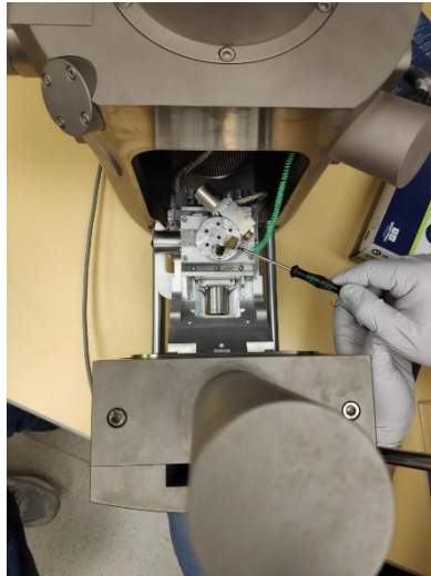
Figure 3.12: Base of SEM – Placement of samples on the base
