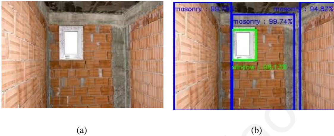
Figure 4.7: Custom OD model implementation (example 3): (a) Initial random photo, (b) Detected objects by custom OD model
